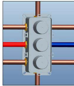
② connect water pipe with installation box
