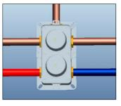
put the installation box in the slot and connect water pipe
