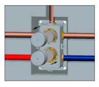
take out the two caps, install handles, do water testing make sure there is no leakage problem
