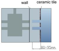
① slotting in the wall the depth of hole is from 80 to 95mm
