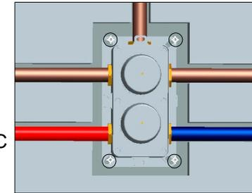
④ put the installation box, and drill holes on the wall, insert the plastic expansible screw
